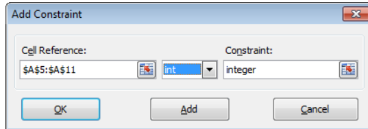
FIGURE 30-3 This constraint defines as an integer the number of workers who start each day.
