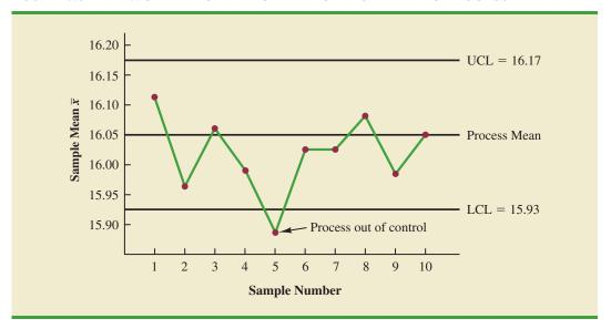
FIGURE 20.6 THE \$\bar{x}\$ CHART FOR THE CEREAL CARTON FILLING PROCESS
